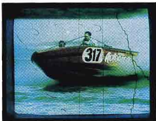
The first photo shows the green tint, which was on the original film. In the middle photo, the excess green has been removed by the automatic color-correction circuitry. However, the scratches still remain. The last photo shows how the dirt and scratch elimination system completely eliminated all traces of scratches from the image. The result of the two circuits is a greatly improved video image.
