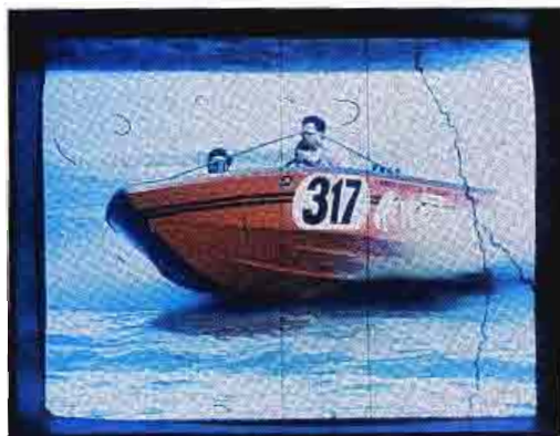
The first photo shows the green tint, which was on the original film. In the middle photo, the excess green has been removed by the automatic color-correction circuitry. However, the scratches still remain. The last photo shows how the dirt and scratch elimination system completely eliminated all traces of scratches from the image. The result of the two circuits is a greatly improved video image.
